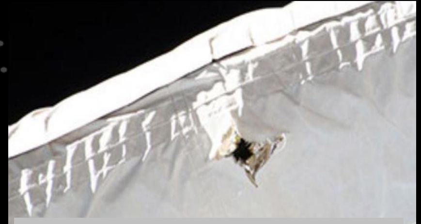
MMOD damage to ISS robotic arm
